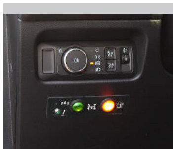
Integrated control panel for Versalift in cabin
