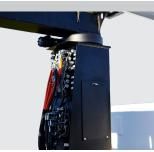
Ground level emergency lowering from the chassis (pedestal mounted valve bank)
